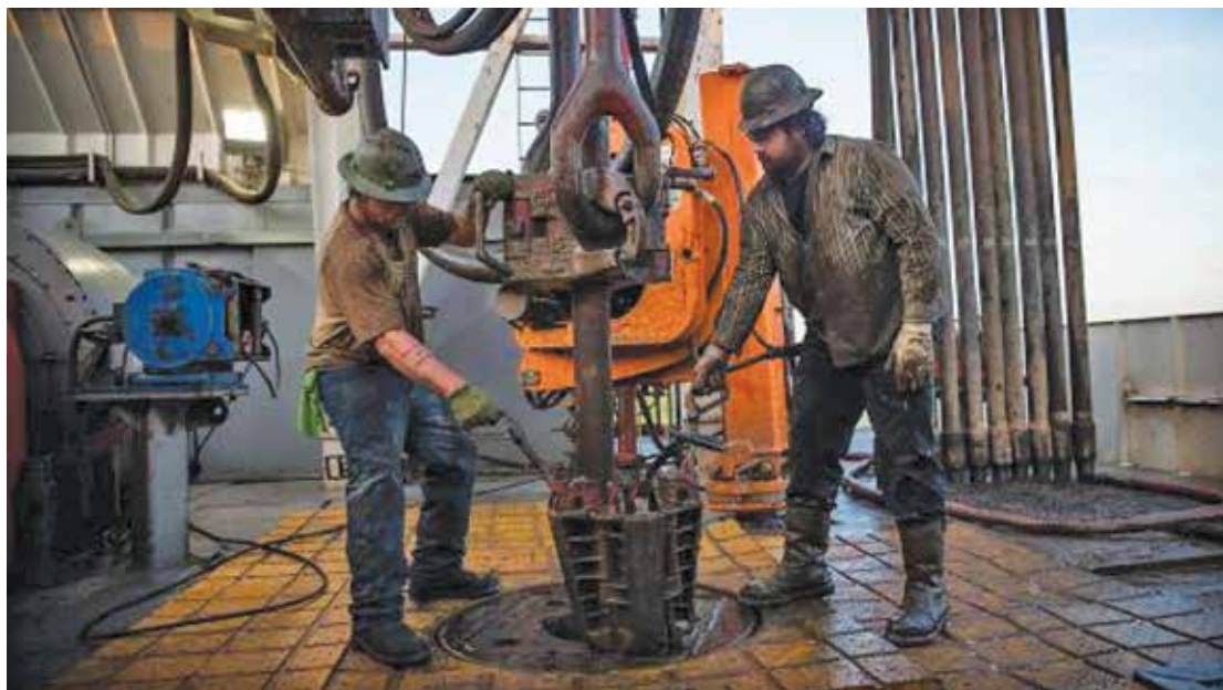
Workers with Raven Drilling line up pipe while drilling for oil in the Bakken shale formation outside Watford City, North Dakota
